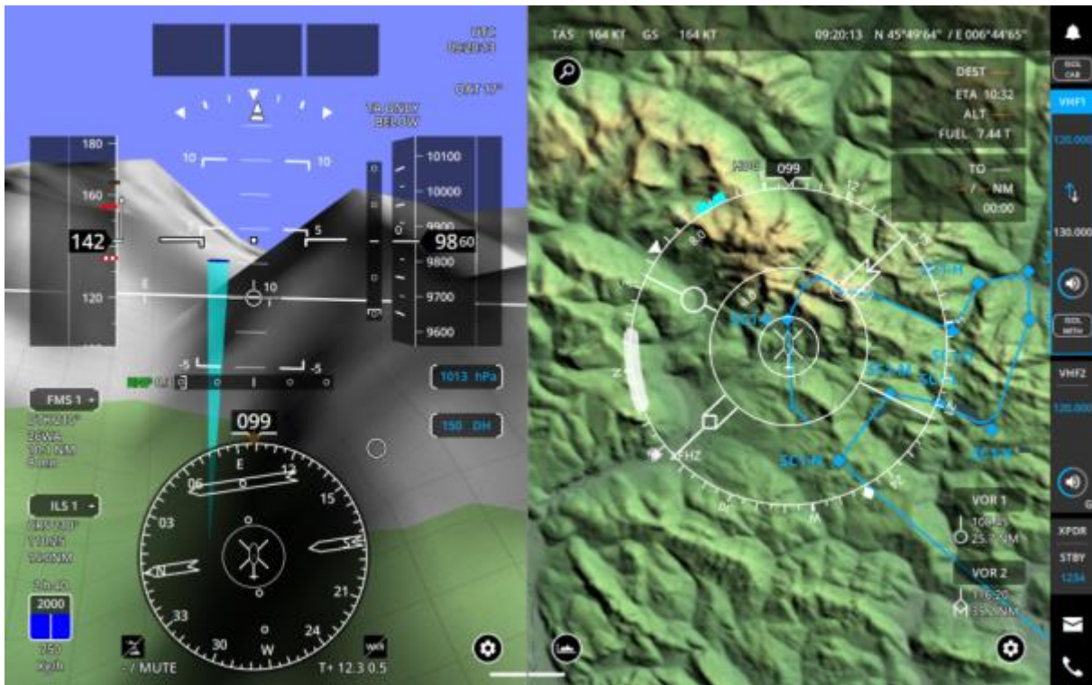
Figure 7: PFD and ND to be displayed on the HDD of the simulator
