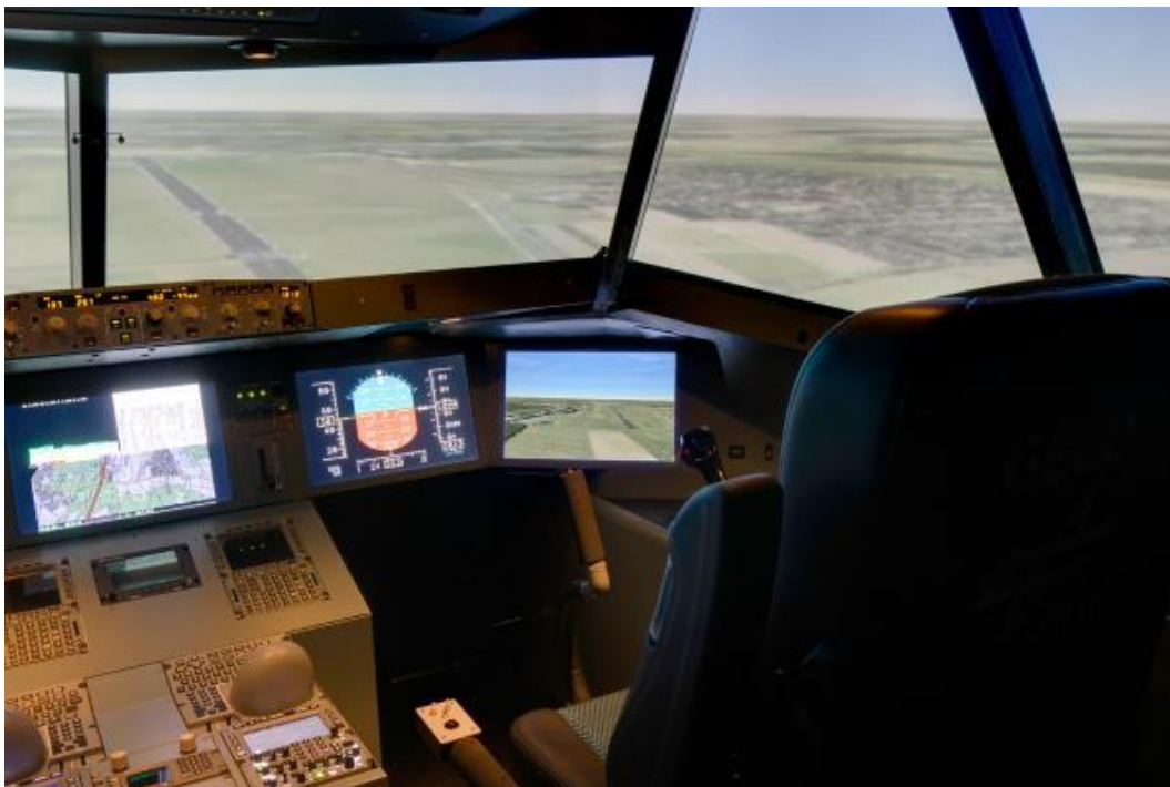
Figure 2: Generic Cockpit Simulator GECO in helicopter configuration at DLR Braunschweig
