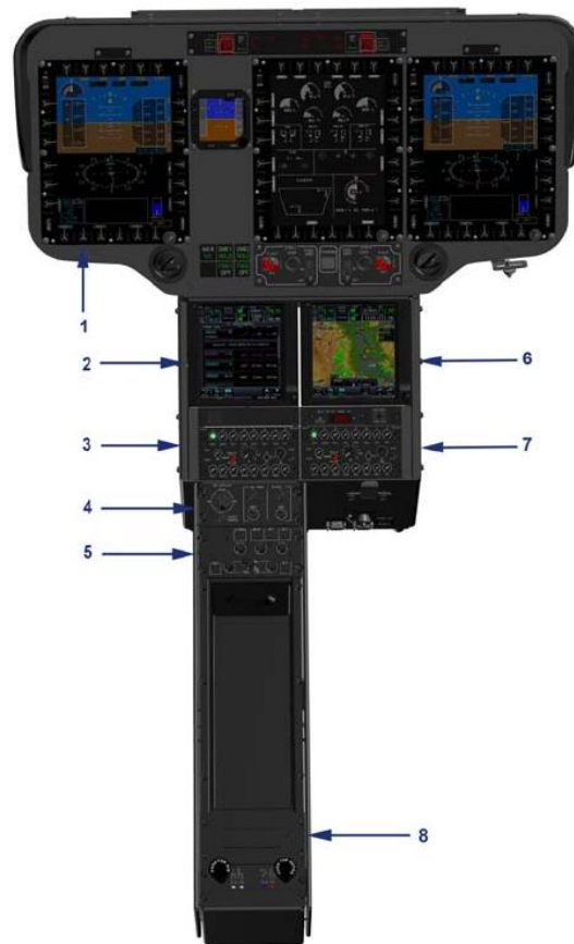
Figure 14: H145 Avionics Layout Single / Dual Pilot IFR with Dual GTN 750
